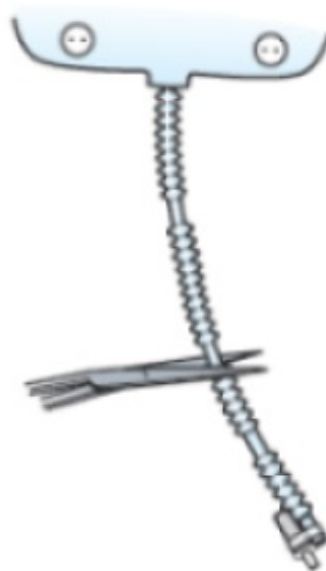
Figure 17. Cut the tubing
