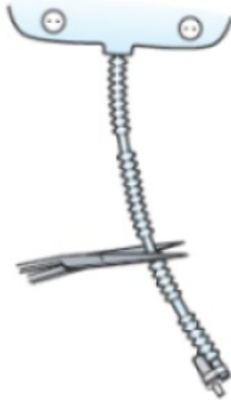
Figure 17. Cut the tubing
