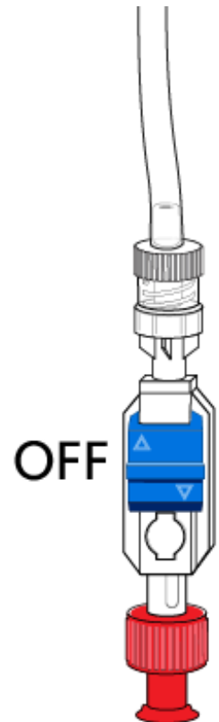
Figure 2. Flow switch and disposable cap
