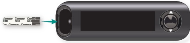
Figure 10. Put the test strip into the port
