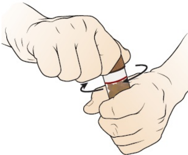
Figure 7. Cap the tube tightly
